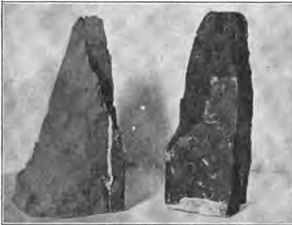
Fig. 31. — Hard Brick in Compression.
